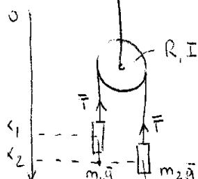
$$\left. \begin{array}{l} l = x_1 + x_2 + IR \\ m_1 \ddot{x}_1 = m_1 g + T \\ m_2 \ddot{x}_2 = m_2 g + T \end{array} \right\} \text{ур-я связи}$$
