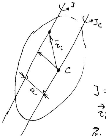
$$\begin{aligned} J &= \sum_i m_i r_{i_1}^2 \\ &\rightarrow \vec{r}_{i_1} = \vec{r}_c + \vec{r}_{ic} \\ &\vec{r}_{i_1} = \vec{r}_{c_1} + \vec{r}_{ic_1} \end{aligned}$$
