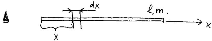
$$x_c = \frac{1}{m} \sum_i m_i x_i \quad m_i \rightarrow dm = \frac{m}{l} dx$$
