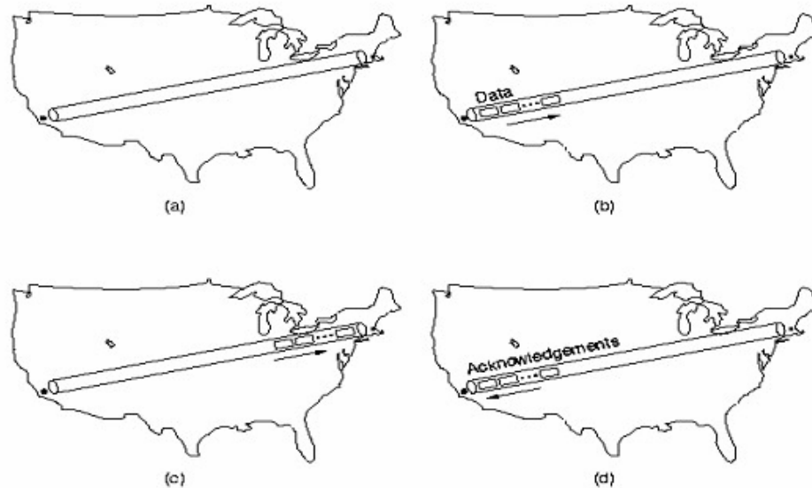
Fig. 6-46. The state of transmitting one megabit from San Diego to Boston. (a) At t = 0 . (b) After 500 \mu\text{sec} . (c) After 20 \text{ msec} . (d) After 40 \text{ msec} .
