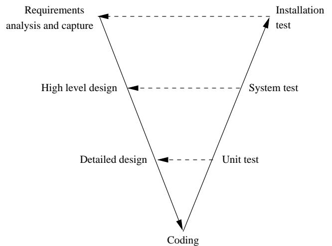
The V-diagram illustrates the typical life-work cycles which we discover errors by testing.
